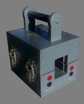
The Conformity Assessment Business Model DCS06 Clamp is designed and tuned for optimal operation in the 100 kHz frequency range and provides efficient coupling of the Defence Standard 59-411 DCS06 pulse to the EUT at voltages up to 1 kV (single turn output) and 4 kV (4 turn output). A single turn monitor loop is provided for pulse amplitude measurement during test.
